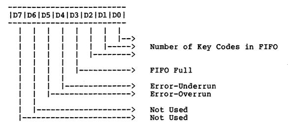
If bit D3 is "1", then the FIFO is full (the FIFO can contain up to eight key codes). The two error conditions which can be detected are underrun and overrun. Underrun occurs when the CPU tries to read data from the Data Register but the FIFO is empty. Overrun occurs when a keyswitch closure is detected but the FIFO is already full. If either error bit is a "1" value, then the corresponding error condition was detected.
