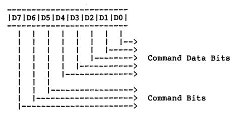
The Command Bits specify the command being issued to the 8279, and the Command Data Bits give the data associated with the command. Only three 8279 commands are used by the system software. The function of each of these commands and the definition of the corresponding data bits is as follows: Keyboard Controller Initialization:
