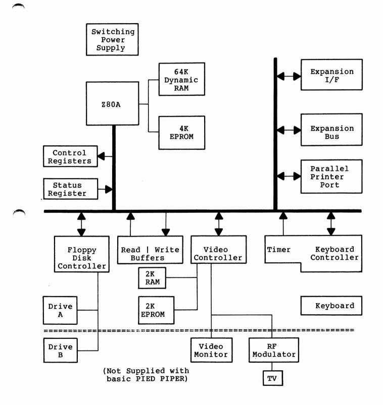
Fig. 2.1 Basic PIED PIPER hardware configuration.
