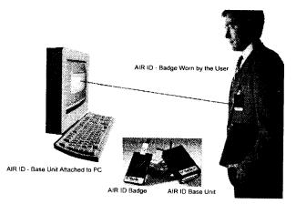
The Base Unit is attached to the serial port using the cable and adapter. The badge may be clipped to the user's belt, jacket, collar, inside front pocket, or worn around the neck.
