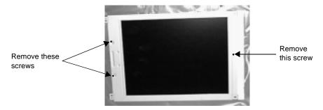
**Note** On early models, the 2 screws on the same side of the display are covered by the gasket. The gasket material covering the two screws must be removed. On later models, the gasket will be notched to allow accessibility to the screws.
