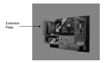
5. Remove the slot cover that corresponds to the extension plate and the appropriate slot on the back-plane board. The cover is secured by a single screw.
