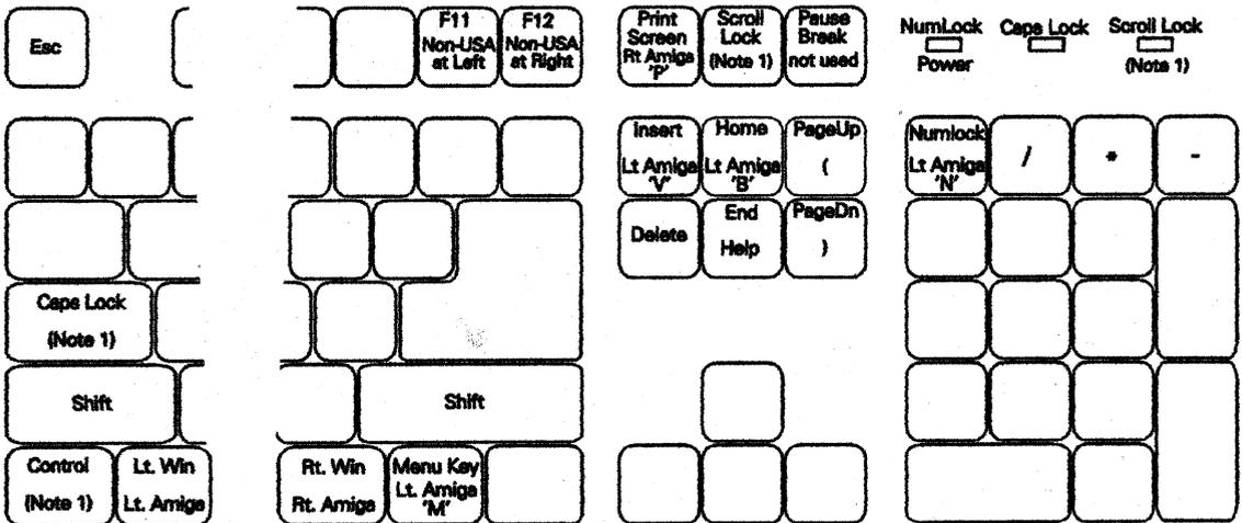
Note 1: Scroll Lock LED ON = PC Style: Caps Lock is Caps Lock and Left Control is Control
