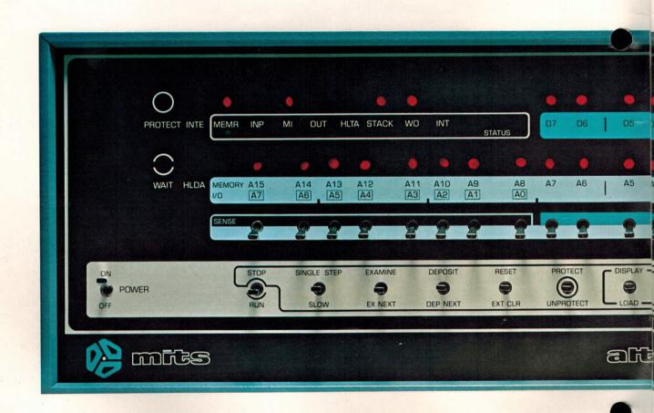
The Display/Control Board features a programmable read only memory (PROM) which contains the program operations for examine, examine next, deposit, deposit next and accumulator functions. The PROM eliminates the need for single-shot control of those functions.
