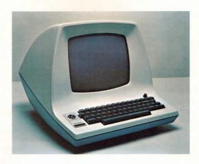
Auxiliary Interfaces: Extension RS-232C port Communication Rates: 75, 110, 150, 300, 600, 1200, 1800, 2400, 4800, 9600, 19,200 baud (switch selectable). Transmit/Receive Modes: Full and half duplex (switch
