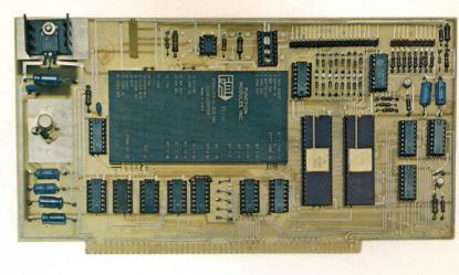
Stability Coefficients: Offset vs. Temperature—20 ppm/°C (max). Gain vs. Temperature—80 ppm/°C (max). Nonlinearity vs. Temperature—20 ppm/°C (max). Gain vs. Supply Voltage—±30 ppm/% Vs (max).
