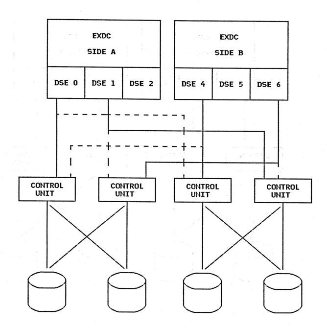
3.17 IEM WASHINGTON SYSTEMS CENTER (C) COPYRIGHT IBM CORP. 1982 IBM 3084 PROCESSOR COMPLEX **3084 CHANNEL CONFIGURATION** SHARED MIXED MODE - PARTITIONED
