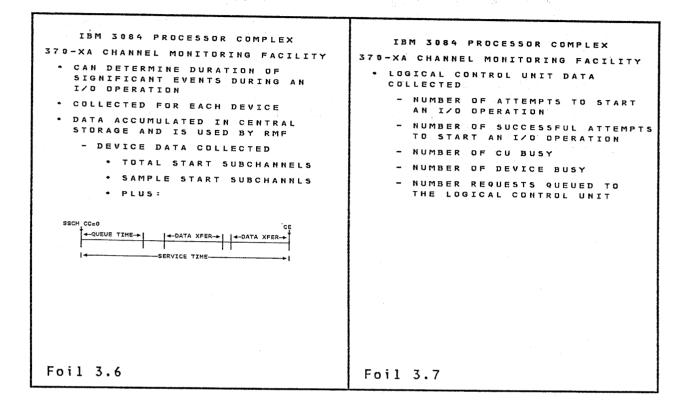
The Channel Monitoring Facility is a timer driven function that provides the ability to determine the duration of significant events that occur during an I/O operation. Data is accumulated on a device basis and is stored in Central Storage. The data will be used by RMF to produce I/O and device related reports.
