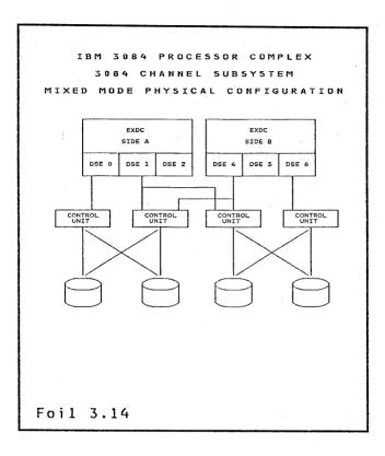
If the 3084 will be run in partitioned mode for any length of time, then four paths, two from each side (EXDC) is probably more appropriate. This provides two paths to all the devices when the system is running in partitioned mode. For example, using the diagram in the above foil, one could physically cable the control units as shown.
