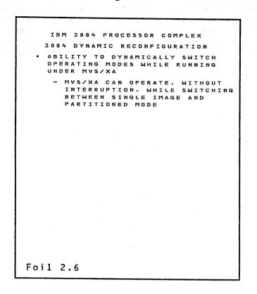
The 3084 is capable of dynamically changing operating modes. This is accomplished by using a series of CONFIGuration commands under MVS/XA<sup>12</sup> and by issuing a VARY PHYSICAL command to the 3082 Processor Controller from the system console. These commands provide the capability of configuring an entire side into or out of a single image mode environment<sup>13</sup>.
