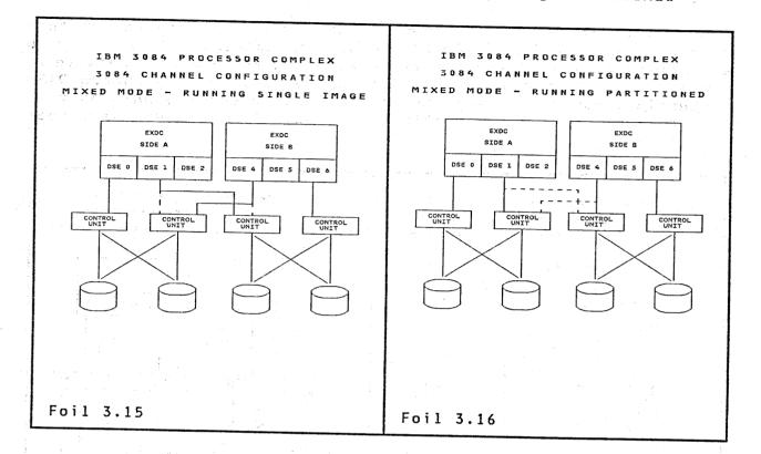
However, when running in single image mode, the path from DSE 1 could be configured offline to the left hand pair of control units, while the path from DSE 4 could be configured offline to the right hand pair of control units. This would give each pair of control units two paths (that's all they would ever need), one path from each EXDC.
