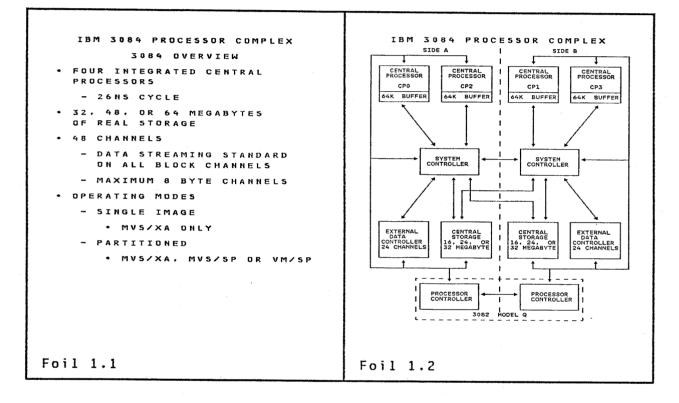
The 3084 is a tightly-coupled processor. It has four integrated central processors. The 3084 is organized into two symmetric sides; Side A and Side B. Each side is essentially a 3081 K Processor. Therefore, the 3084 can be viewed as being the result of merging two 3081 K systems.
