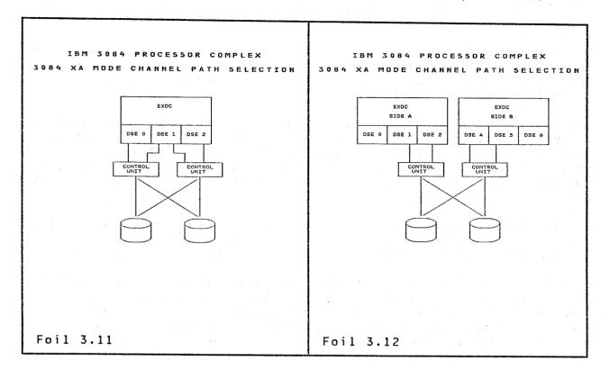
The intent of these two foils is to illustrate how 370-XA path selection works with a single EXDC and how it works with two EXDCs. These foils are not intended to suggest how channels should be configured. Channel configurations will be covered later in this section.
