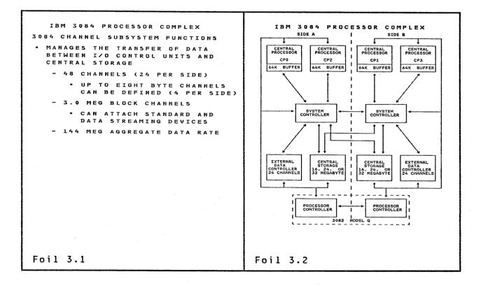
The 3084 channel subsystem manages data transfer between the I/O control units and Central Storage. The functions provided include the following:
