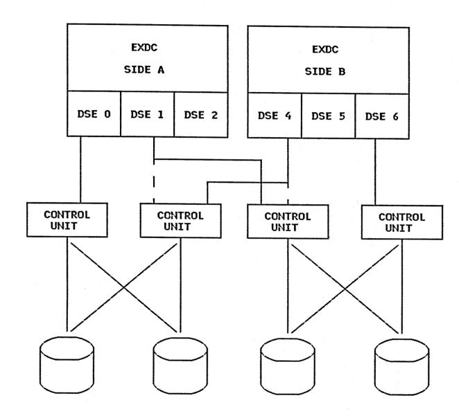
IBM 3084 PROCESSOR COMPLEX **3084 CHANNEL CONFIGURATION** MIXED MODE - RUNNING PARTITIONED
