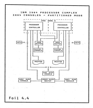
In partitioned mode, the programmable switches are set by the 3082 microcode so that each system console is attached to its side only. This establishes a configuration exactly like a stand alone 3081 K.
