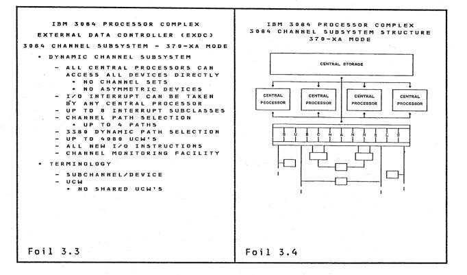
The following is a review of the capabilities of the 3084 channel subsystem operating under MVS/XA.
