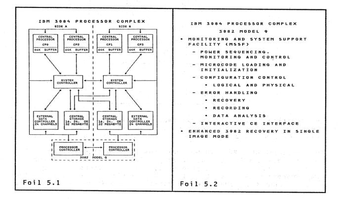
The 3082 Model Q Processor Controller (PC) provides monitoring and system support functions for the 3084 Processor<sup>20</sup>. The 3082 Q is essentially a combination of two 3082 Model 24s. When operating in single image mode, one half of the 3082 Q, usually Side A, is active, while the other half is in standby mode. In partitioned mode, each half of the 3082 Q supports the side to which it is attached.
