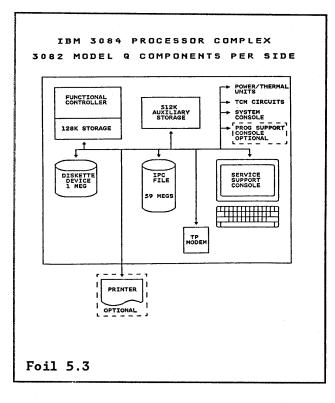
Before getting into the details of how the 3082Q operates, it may be worthwhile to review the 3082Q components and their functions.
