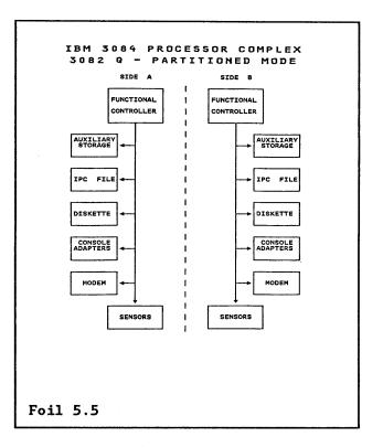
In partitioned mode, the 3082Q is split into two independent sides. Each side is equivalent to a 3082 Model 24. Each side is powered separately. So that when running partitioned, one side could be powered down without effecting the other side.
