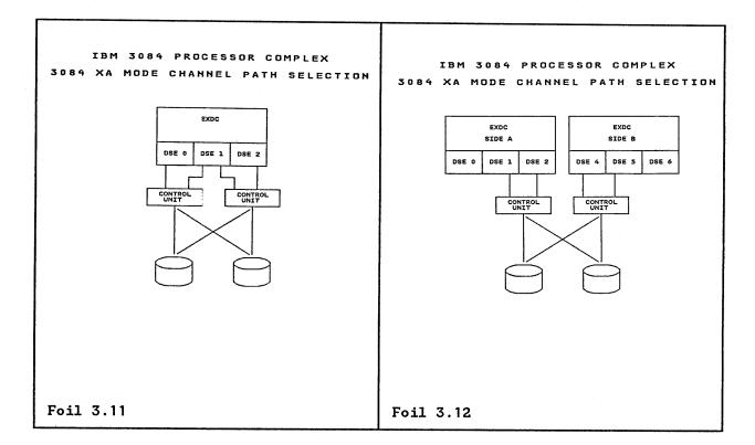
The intent of these two foils is to illustrate how 370-XA path selection works with a single EXDC and how it works with two EXDCs. These foils are not intended to suggest how channels should be configured. Channel configurations will be covered later in this section.
