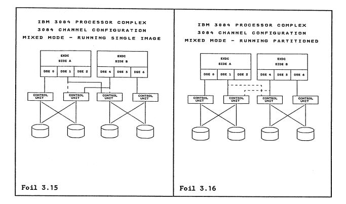
However, when running in single image mode, the path from DSE 1 could be configured offline to the left hand pair of control units, while the path from DSE 4 could be configured offline to the right hand pair of control units. This would give each pair of control units two paths (that's all they would ever need), one path from each EXDC.
