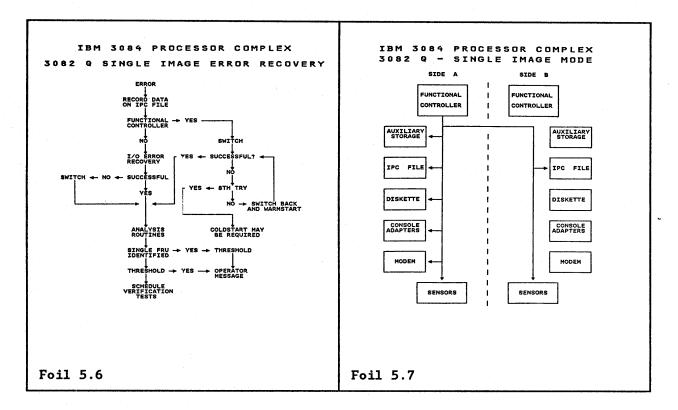
As you can see, all components of the 3082Q, except the inactive functional controller, are connected to the active functional controller. All components of the 3082 have backup except the sensors. Because the sensors are wired to each side, both sets of sensors must be operational. A failure of either sensor is a catastrophic failure and will require an IML.
