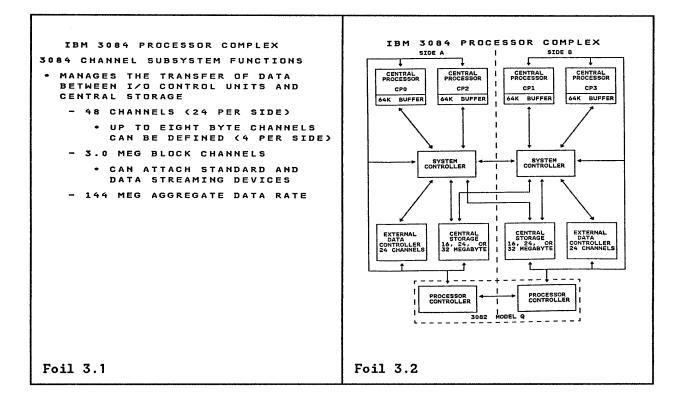
The 3084 channel subsystem manages data transfer between the I/O control units and Central Storage. The functions provided include the following:
