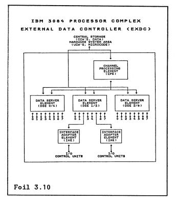
When the 3084 is running in single image mode under MVS/XA, the channel subsystem is logically the same as it is on any 308X system. That is, any central processor has direct access to any I/O device. And any processor can field an I/O interrupt whether or not that processor initiated the I/O operation. The difference on the 3084 is that it has two EXDCs. Therefore, the microcode will work slightly different.
