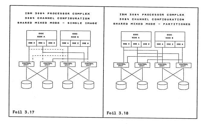
As you can see, this physical configuration is slightly different from the previous configuration in that there are two physical paths to each control unit. When running in single image mode, one path to each control unit is configured offline in such a way as to provide a path from each EXDC to each pair of control units.
