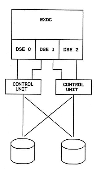
IBM 3084 PROCESSOR COMPLEX 3084 XA MODE CHANNEL PATH SELECTION
