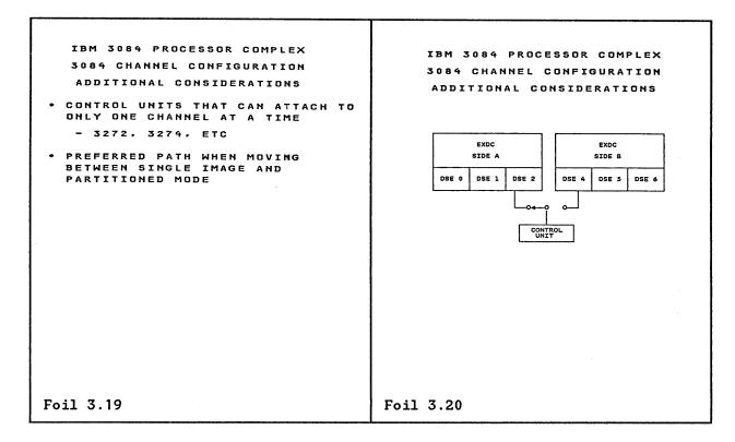
Although asymmetric devices (as relates to processor affinity) do not exist in 370-XA mode, an installation must still concern itself with devices that have control units that can attach to only one channel at a time, e.g., 3274. For these kinds of devices a switch, such as the 3814, should be used so that the device can be switched to another path. Again, if running predominately in single image mode, this second path should be from the other EXDC.
