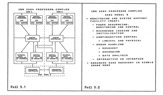
The 3082 Model Q Processor Controller (PC) provides monitoring and system support functions for the 3084 Processor<sup>18</sup>. The 3082Q is essentially a combination of two 3082 Model 24s. When operating in single image mode, one half of the 3082Q, usually the A-side, is active, while the other half is in standby mode. In partitioned mode, each half of the 3082Q supports the side to which it is attached.
