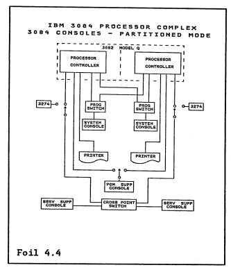
In partitioned mode, the programmable switches are set by the 3082 microcode so that each system console is attached to its side only. This establishes a configuration exactly like a stand alone 3081K/KX.
