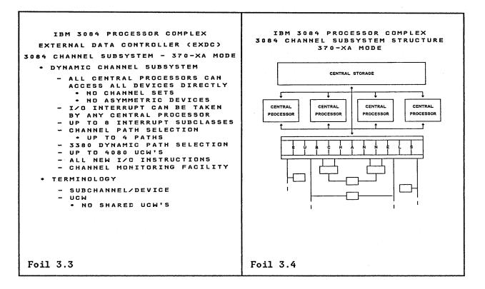
The following is a review of the capabilities of the 3084 channel subsystem operating under MVS/XA.
