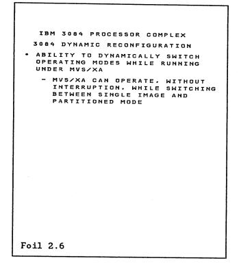
The 3084 is capable of dynamically changing operating modes. This is accomplished by using a series of CONFIGuration commands under MVS/XA<sup>11</sup> and by issuing a 'vary physical' (VARYPHY) command to the 3082 Processor Controller from the system console. These commands provide the capability of configuring an entire side into or out of a single image mode environment<sup>12</sup>.
