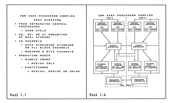
The 3084 is a tightly-coupled processor. It has four integrated central processors. The 3084 is organized into two symmetric sides; the A-side and the B-side. Each side is essentially a 3081K/KX Processor. Therefore, the 3084 can be viewed as being the result of merging two 3081K/KX systems.
