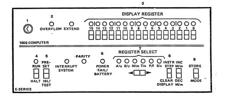
FIGURE 3-1 HP21MXE COMPUTER FRONT PANEL, CONTROLS AND INDICATORS
