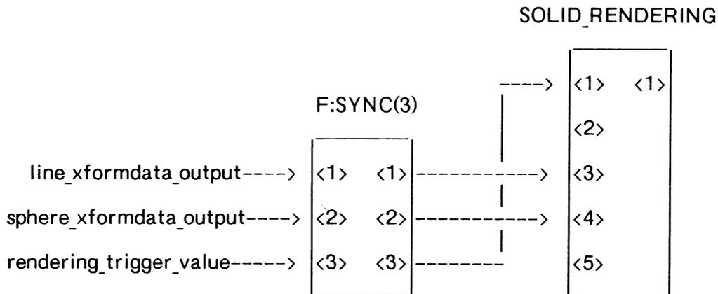
The second potential timing problem deals with the triggering of F:XFORMDATA. An instance of F:XFORMDATA must not be triggered while it or any other instance of F:XFORMDATA is still active. Thus when using multiple instances of F:XFORMDATA, one instance should be used as the trigger for the next. (See the following example.)
