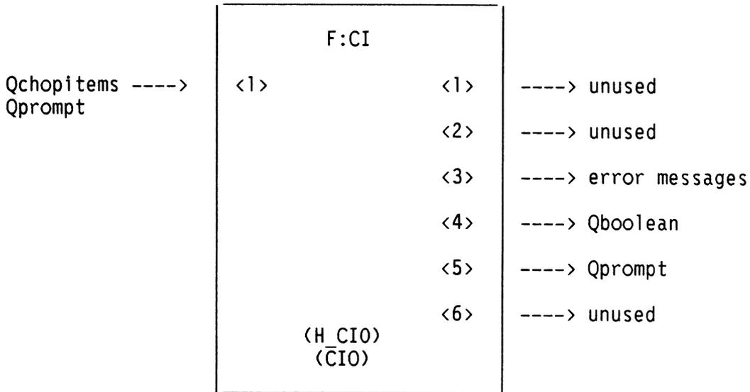
This function interprets commands, creating display structures and function networks. It receives input either from a chop/parse function or a Readstream function (if using the GSRs).
