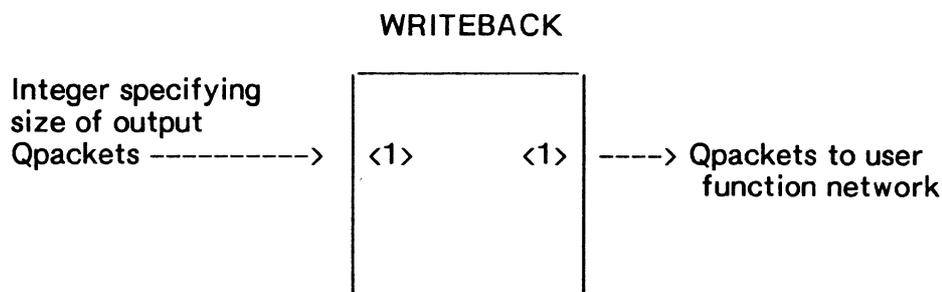
WRITEBACK sends encoded writeback data received from the display processor. The writeback data is prefixed by a start-of-writeback command, followed by the encoded data, followed by an end-of-writeback or end-of-frame command.
