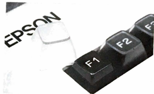
The removable keycaps on the ASCII keyboard function keys. Custom legends can be inserted under the keycaps.
