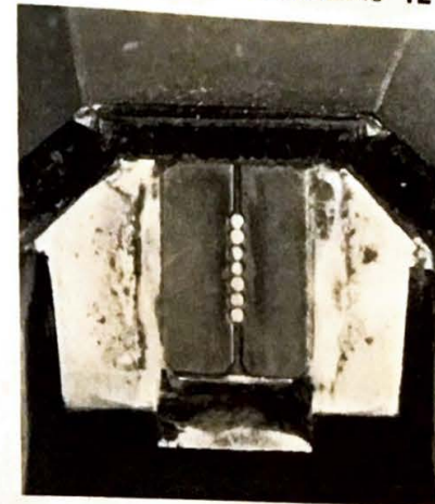
The print wires of a dot matrix printer head. The wires are typically about .012 inches in diameter. This particular head was used in an old Centronics printer.
