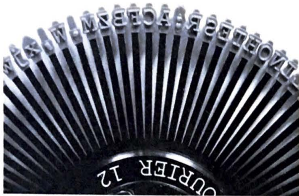
The typing element used in daisy wheel printers.
