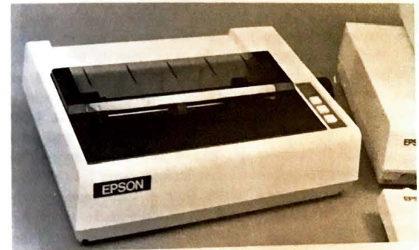
The legendary MX-80 printer from Epson. This printer can be used with Valdocs, but does not have down-loadable fonts or proportional spacing available in the Valdocs editor.
