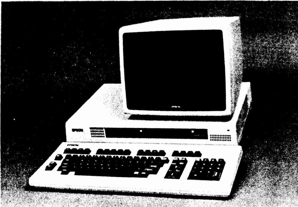
The Epson QX-10 computer shown with the HASCI keyboard.
