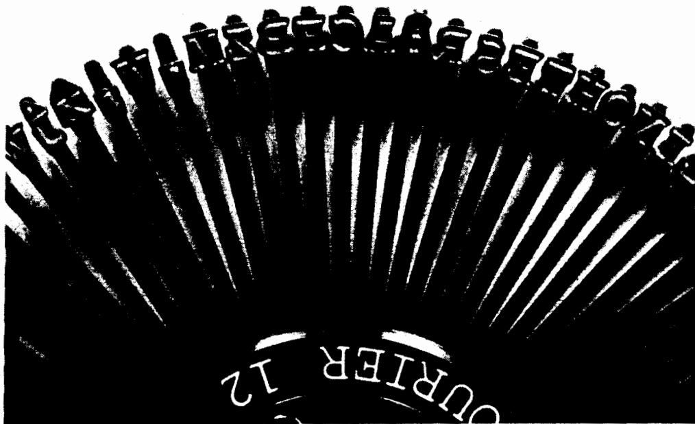
The typing element used in daisy wheel printers.
