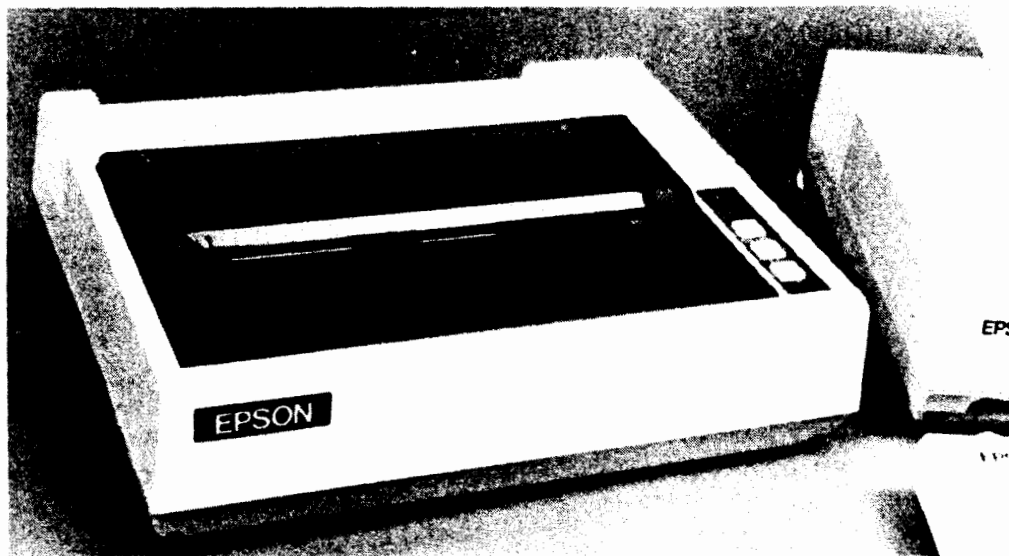
The legendary MX-80 printer from Epson. This printer can be used with Valdocs, but does not have down-loadable fonts or proportional spacing available in the Valdocs editor.
