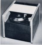
the stylus assembly and turntable, power supply, input interface and search logic, readout and errorcheck electronics, and output interface. It is 9" high, 10<sup>1</sup>/<sub>2</sub>" wide, 12" deep, weighs 30 pounds, and draws less than 0.75 amp at 115 VAC.
