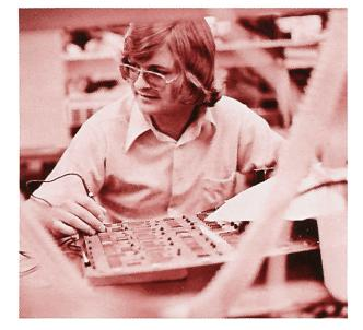
*Incoming Test:* The components we buy are stringently tested as they come in. That includes integrated circuits, transformers, peripherals, circuit boards, castings, pieces of hardware and sheet metal.
