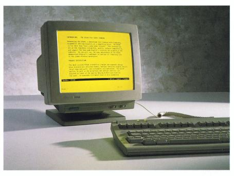
The VT420 text terminal has  $800 \times 414$  pixel resolution, a 70 Hz refresh rate and overscan.
