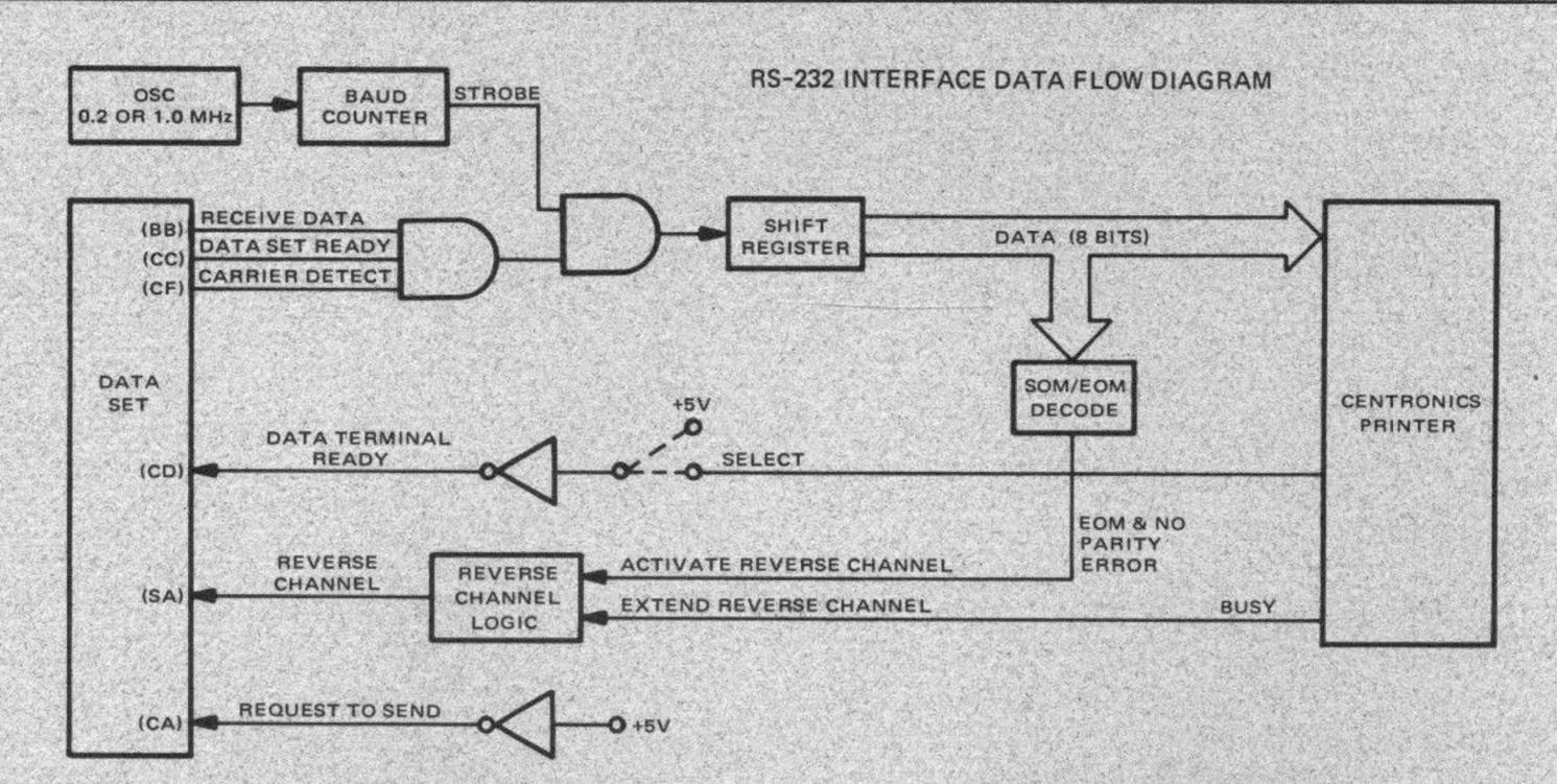
activated by a new EOM for another 200 milliseconds. This delay is generated on the interface board. As a result, new data should not be transmitted for at least 200 milliseconds after Reverse Channel goes inactive.
