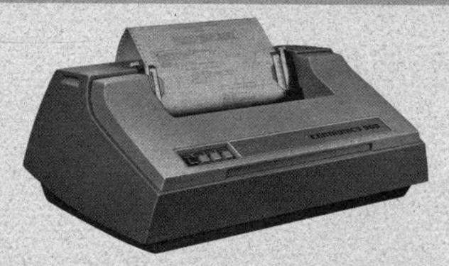
The 500 is a low cost 100 character per second 5 x 7 dot matrix, serial, impact printer that establishes a new price/performance standard. A wide range of options allows the printer to be styled for specific application requirements. Capable of producing an original plus up to four clear carbon copies, the 500 can operate with the paper supply located to the rear or below the printer.
