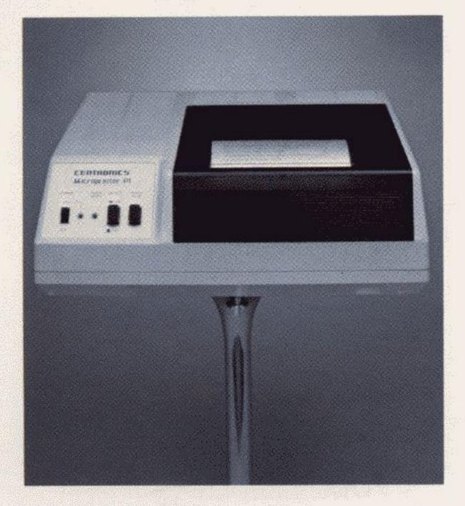
The Centronics P1 Microprinter is a desktop high-speed non-impact printer. It employs state-of-the-art non-impact discharge technology to electrosensitively form characters on coated paper (readily available from Centronics and other sources) with exceptional clarity. Because it prints without impact, it's far quieter than conventional printers.
