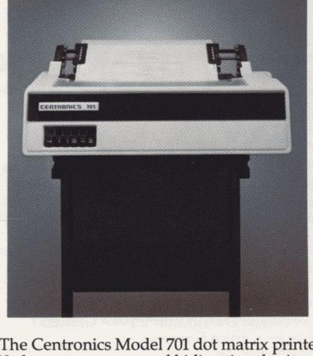
The Centronics Model 701 dot matrix printer is a 60 character-per-second bidirectional printer that offers increased throughput by intelligently seeking the nearest character of the next print line (logic-seeking), thus eliminating time consuming carriage returns.
