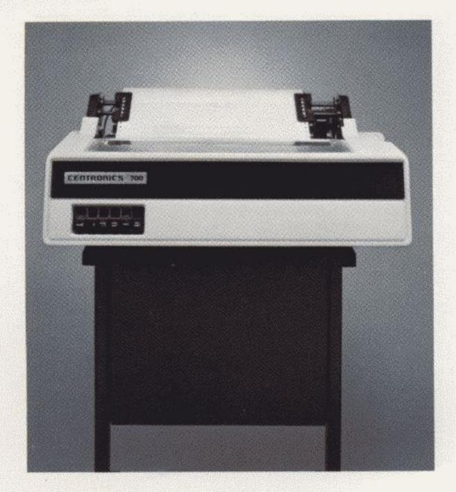
The Centronics Model 700 dot matrix printer is designed for applications that require low throughput (13 to 90 lines per minute) of hard copy output. Its ideal applications include: CRT output, instrument data logging, stand-alone business systems, off-line selective printing, and other areas where high throughput is not required.
