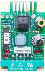
This configuration allows you to play files off the PC directly in to the C64 without recording them to tape.
