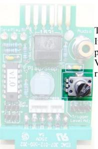
The potentiometer is used to adjust the trigger threshold. It is pre-set to 1.5V with a nail polish marker at that position.
