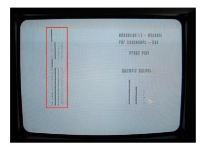
This one shows when the trigger point is wrong (adjust the trigger pot or audio level). You can see there is numerous random lines indicating the trigger is not occurring on each bit pulse but maybe several times.
