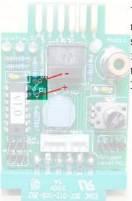
You can measure the trigger threshold voltage with a DC multi-meter, place the negative and positive leads where shown in the picture (careful not to touch the IC pins), aim for about 1.5V to 2.0V, but depending on your sound card this may need to be lower, but generally no higher than 2.0V. For my PC I have this set to 1.6V.
