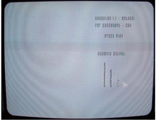
Below is the pattern we are aiming for when the header or ROM loader is playing in to Cassadapt (using WAV-PRG). Three distinct lines just like the picture on the right of the screen with no (or minimal) noise in between the lines.
