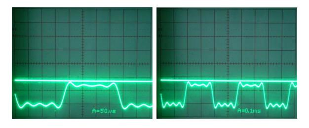
Because the audio never crosses the trigger level there is no output produced for the C64.
