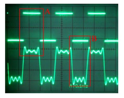
This is what you are aiming for, a perfect conversion of the audio signal to the 0-5V digital signal the C64 requires (in this case a .tap file playing out the sound card of the PC).
