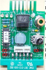
This configuration will allow you to record on to a Datassette from a file playing from the PC (.wav, .tap, .prg etc).
