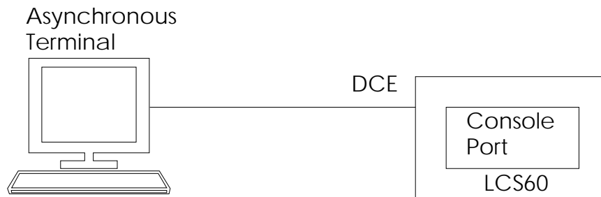
Figure 2-3: System Console Connections – Direct
