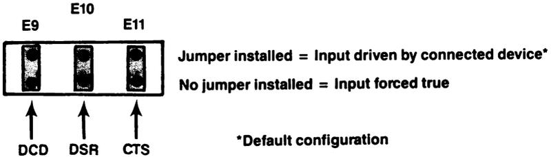
**Figure A-7. Serial Port Input Configuration.**
