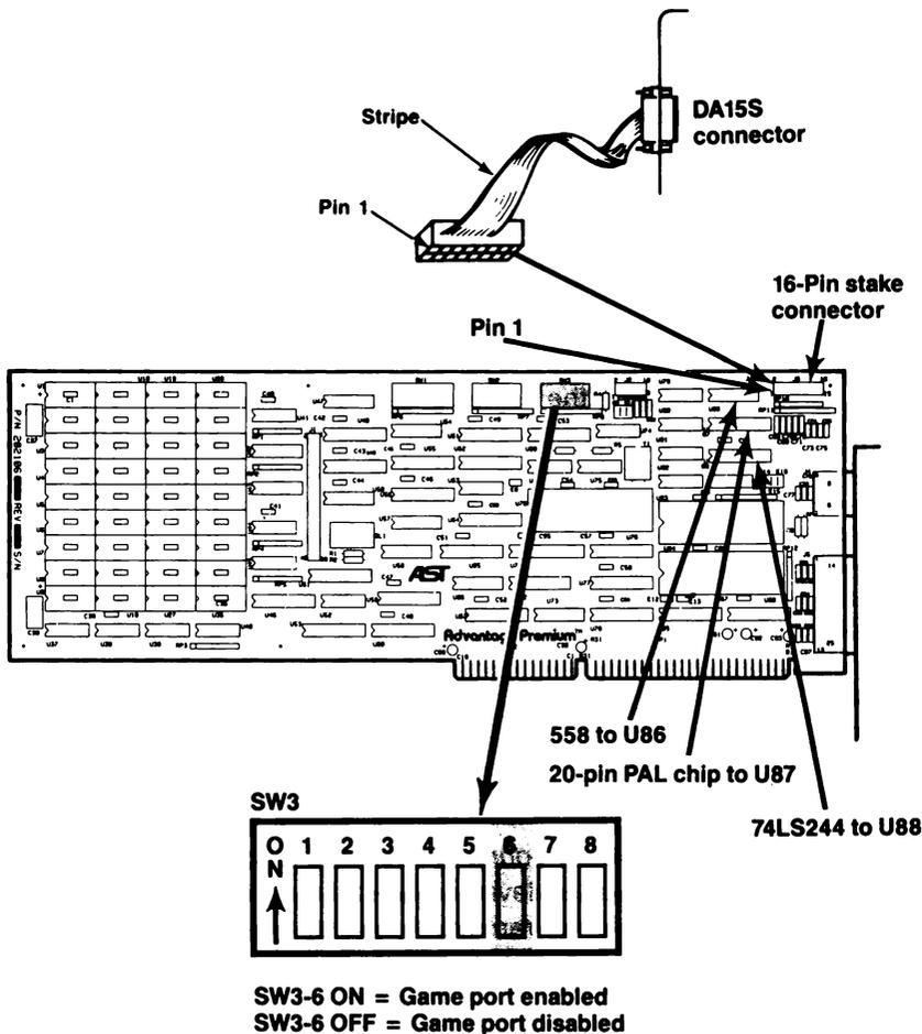
**Figure 7-2. Installing the Game Port Chips.**
