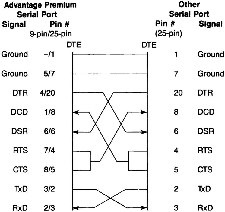
**Figure D-2. Example #1: Null Modem (DTE-to-DTE) Interface.**
