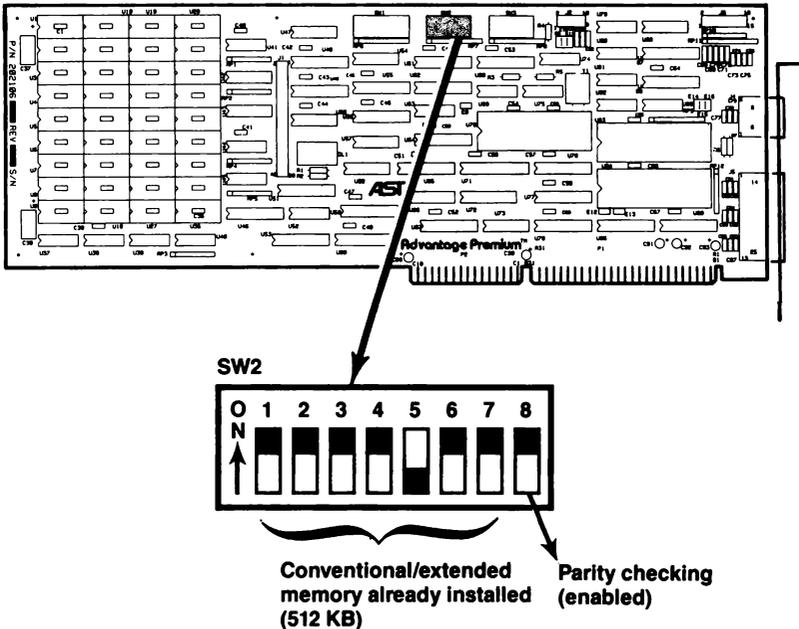
**Figure 2-4. Advantage Premium Switch SW2 (Default Setting).**
