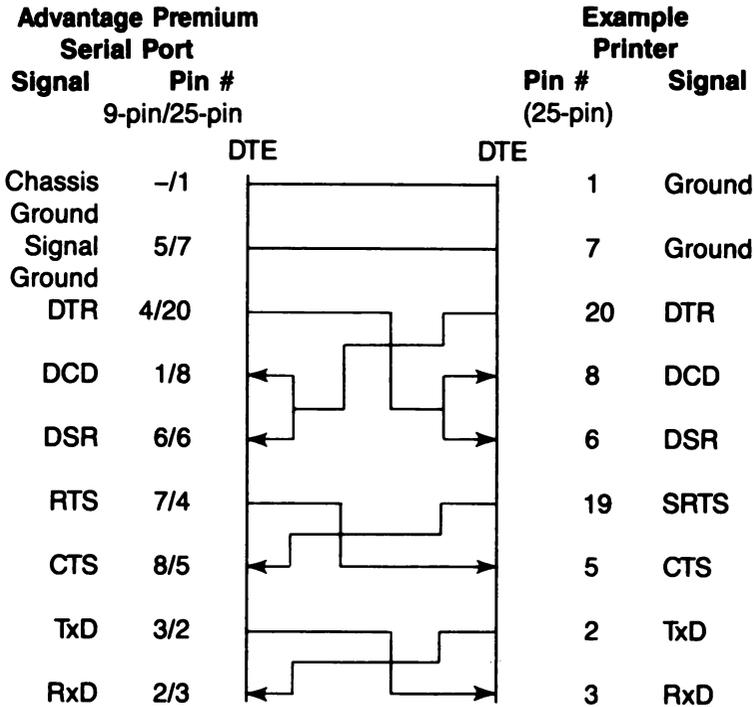
In this case, the printer uses SRTS (Secondary Request to Send, pin 19) instead of pin 4 (RTS); apart from that exception, Figure D-3 follows the ideal DTE input and sequence rules.
