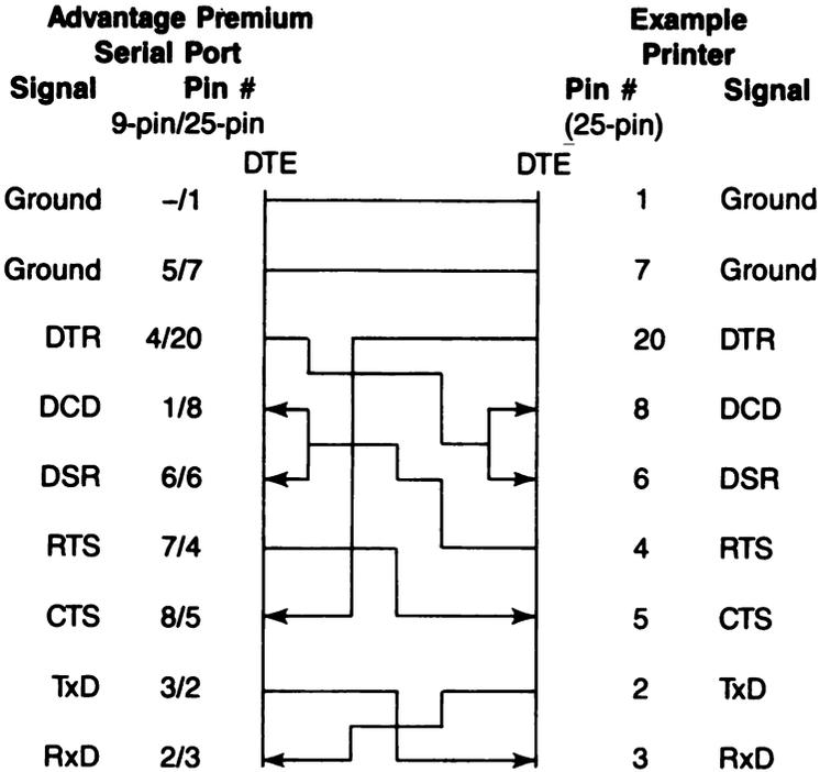
**Figure D-3. Example #2: Null Modem Interface.**
