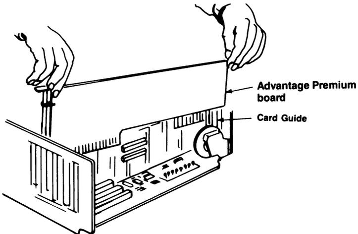
**Figure 3-7. Installing the Advantage Premium Board.**
