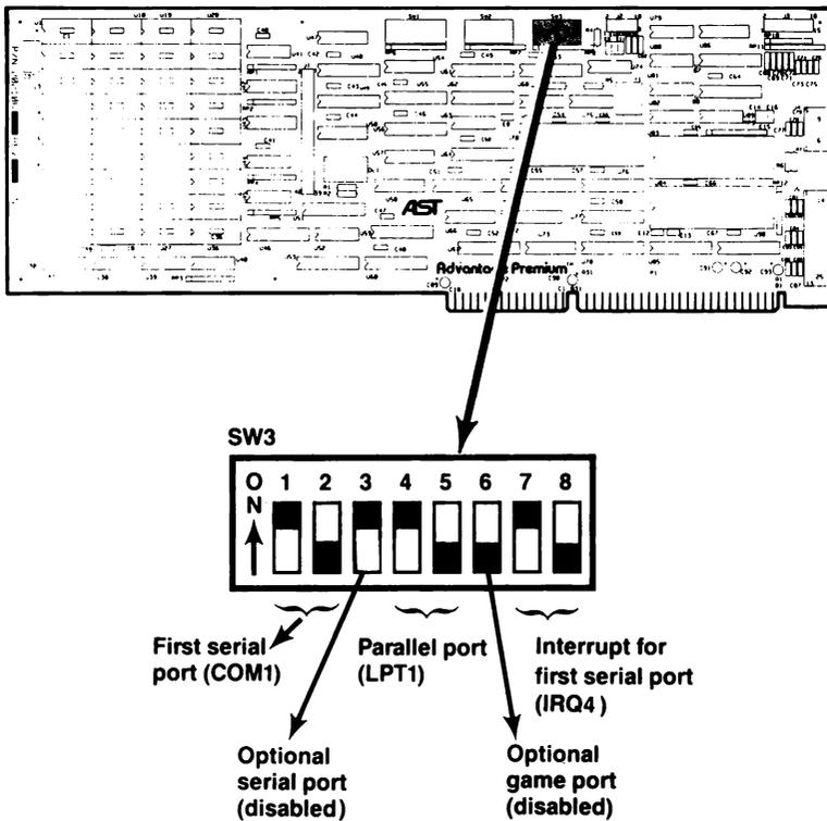
**Figure 2-6. Advantage Premium Switch SW3 (Default Setting).**
