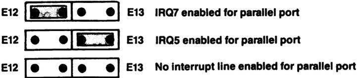
**Figure 6-1. Parallel Port Configuration.**
