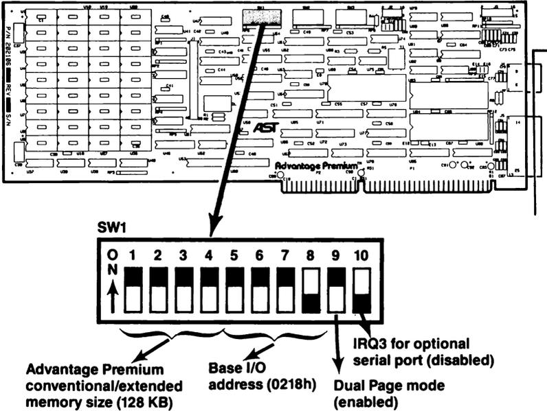
**Figure 2-3. Advantage Premium Switch SW1 (Default Setting).**
