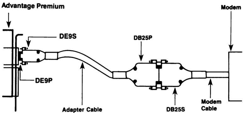
**Figure 5-6. Typical DE9-to-DB25 Cable Application.**
