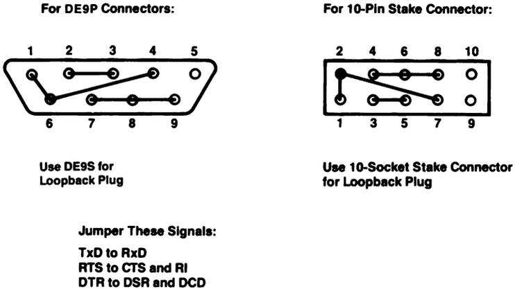
**Figure 5-7. Loopback Plug Configuration.**
