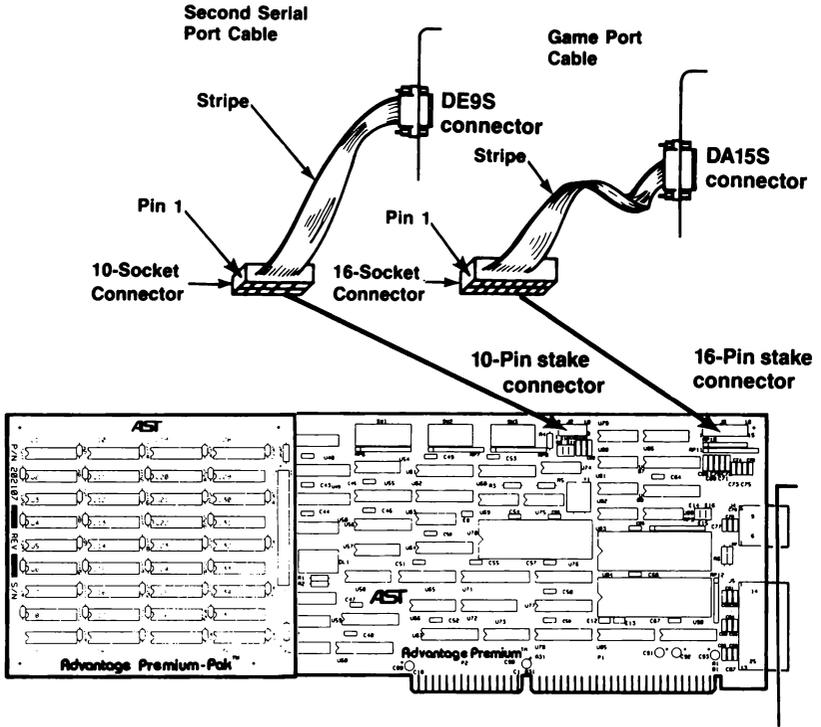
Figure 3-6. Connecting Advantage Premium Cables.
