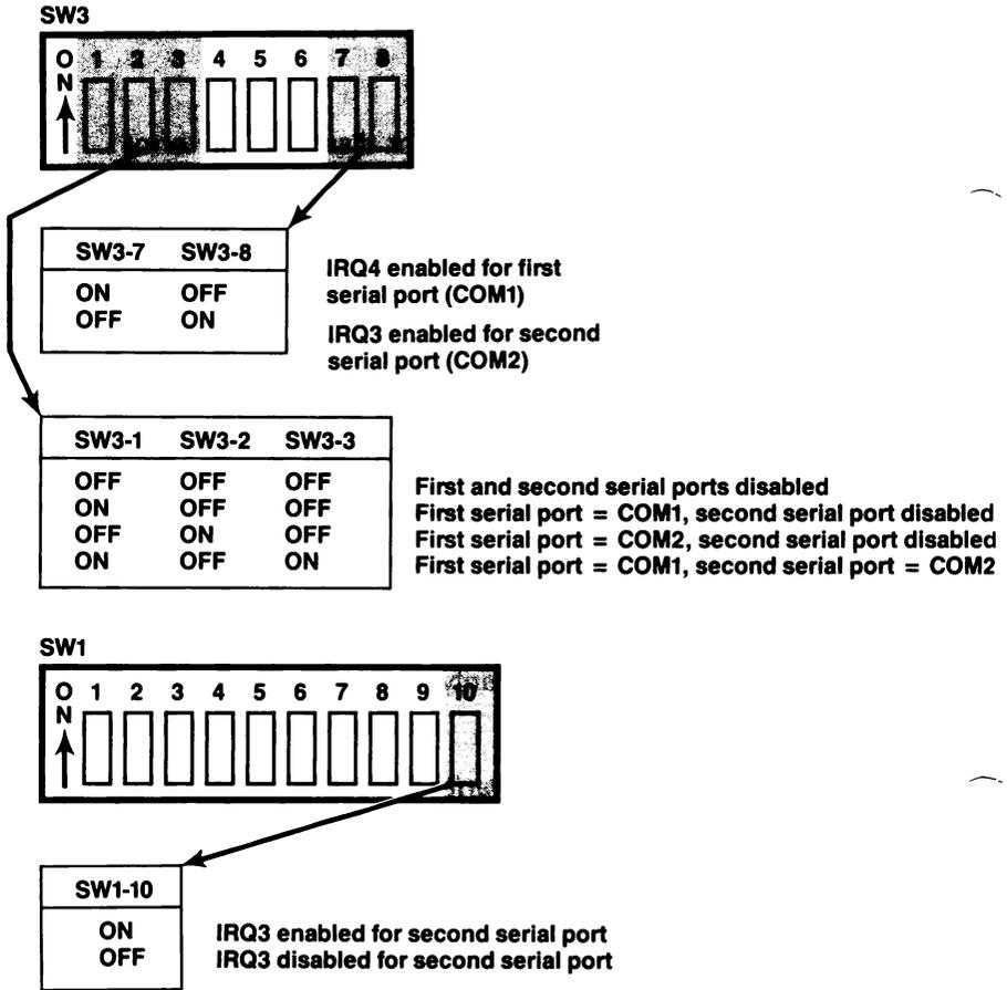
**Figure A-6. Serial Port COM Assignments.**
