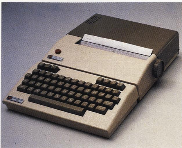
**Package 83** is designed to communicate with destinations on either Telex I or International Telex networks using F1/F2 analog lines. The optional, field-installable IRC Telex kit allows connection to IRC Telex lines. It consists of a Model 1483 teleprinter and a Model 1446 Intelligent Keyboard.
