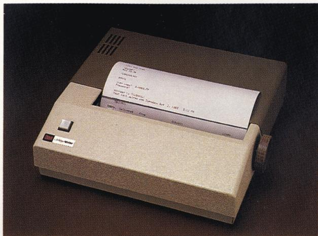
**Model 1980** is an 80/136-column display teleprinter with a Bell 103 compatible internal modem. It connects to public telephone lines (PSTN) in North America as well as to the TWX network. It can be used in messaging, remote computing and TWX compatible applications. Its memory can store and automatically pulse dial up to four phone numbers and log-on sequences required to communicate with remote computers on terminals.
