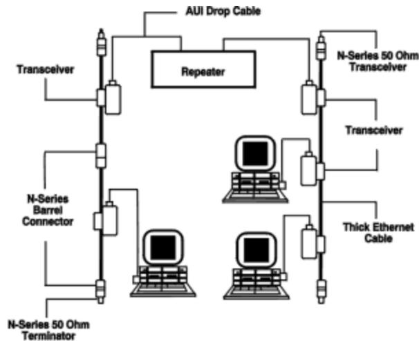
Figure 29: Thick Ethernet Network
