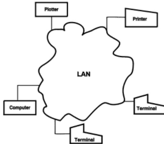
Figure 26: Data Equipments Connected By a LAN
