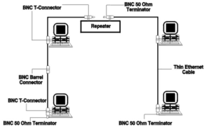
Figure 30: Thin Ethernet Network
