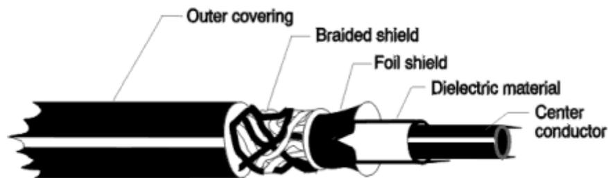
*Figure 8: Detailed Illustration of Segment of Coaxial Cable*
