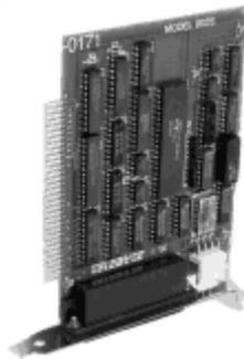
*Figure 22: Low Cost Data Line Analyzer*
