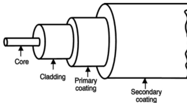
Figure 10: General Structure of Fiber Optic Cable
