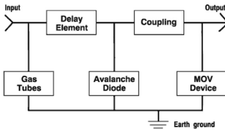
Figure 20: Architecture of a Robust Protection Device
