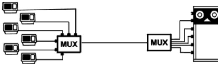
Figure 12C: Terminals sharing a single cable to multi-user computer by multiplexing
