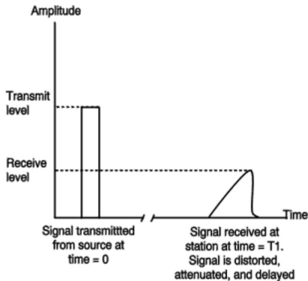
*Figure 9: Illustration Showing Mutual Capacitance and Attenuation Significantly Corrupting a Transmitted Signal on Coaxial Cable*
