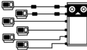
Note: All Terminals Use Short Haul Modems to Support Cable Lengths in Excess of 50 Feet
