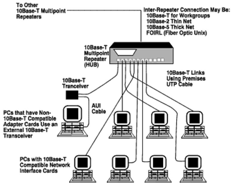
Figure 32: Connecting To An Ethernet LAN
