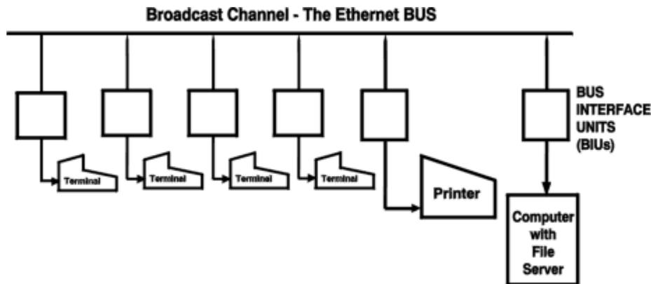
Figure 27: Ethernet Bus Architecture
