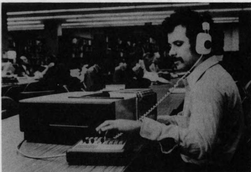
Fig. 1-5. A desktop reading machine (courtesy of Kurzweil Computer Products).
