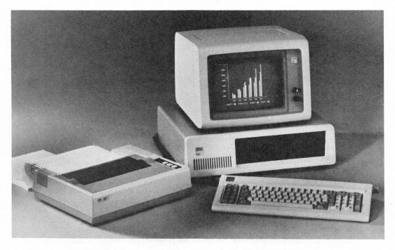
**Figure 1–1** The IBM Personal Computer in a system configuration composed of the monochrome display, keyboard, 80-character matrix printer, and system unit, with two diskette drives installed.
