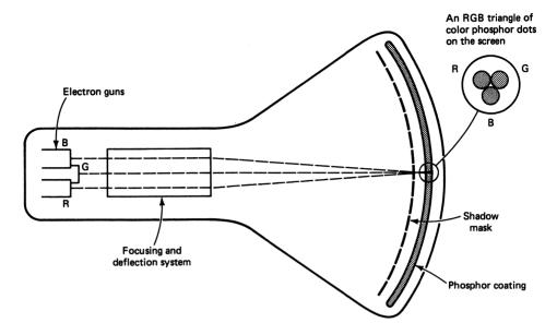
**Figure 1-5** Shadow-mask CRT. Three electron guns, arranged in a pattern to coincide with the arrangement of each triangle of color dots on the screen, are directed onto the dot triangles by a shadow mask. The mask allows only the electrons from the B gun to strike the B dot, the R gun to strike the R dot, and the G gun to strike the G dot.
