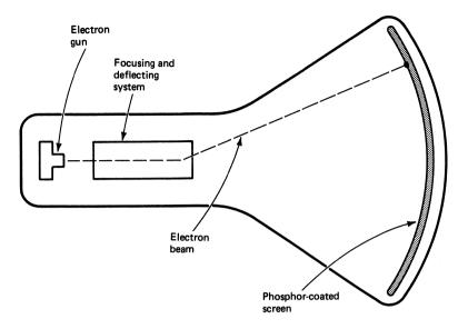
Figure 1-4 Basic operation of a CRT.
