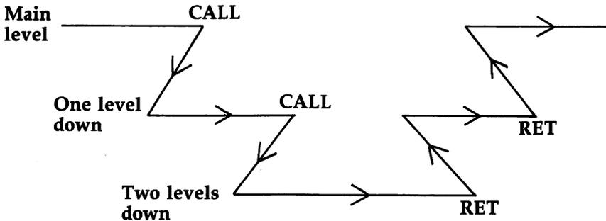
The *near CALL*, or a *Direct Intra Segment CALL*, is much like a near JMP, in that the operand is a 16-bit displacement to the called label. The actual calling mechanism works this way: The IP (Instruction Pointer) register is pushed onto the stack, then the new IP is calculated by adding a displacement to the original IP. Program execution continues at this new position. Since this instruction alters only the IP, you cannot move from one segment to another.
