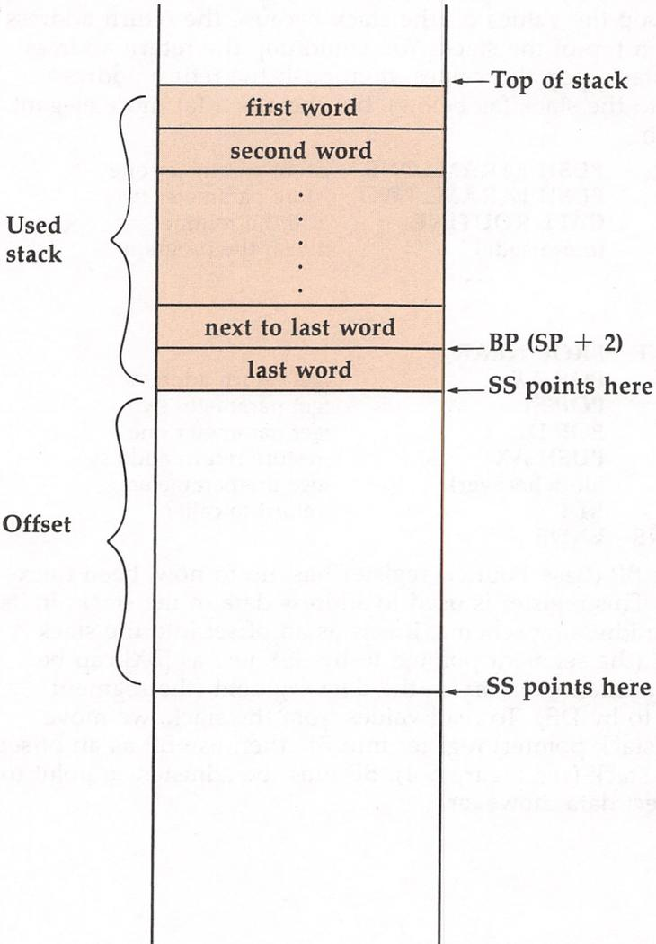
As you can see from Figure 6-4, after moving SP into BP we must add two to BP to address the last word stored on the stack. Remember, the stack grows downward, from higher memory locations to lower ones. For each additional word, we must increment BP by two (if the addressing modes have you confused, be patient; they are all explained in the next chapter). Now examine the code below:
