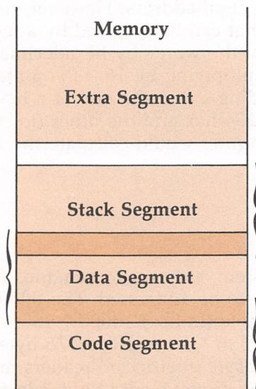
in memory. Using a register is always faster than using data in memory, because registers are, in a sense, part of the 8088. Furthermore, less space is used in program memory to specify one register out of, perhaps, eight, as opposed to one address out of 65,536.
