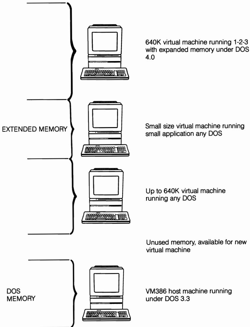
**14-2** Under VM386, isolation is so total that each virtual machine runs under its own copy of DOS. Under certain circumstances, virtual machines can even concurrently run under different (even non-DOS) operating systems. All VMs run entirely in protected mode and cannot crash other VMs or the total system.
