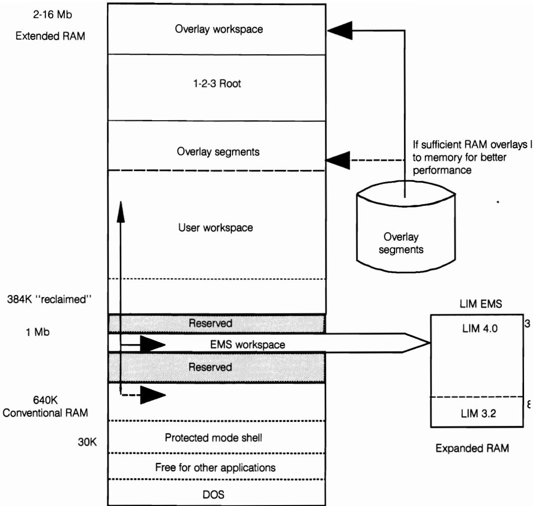
**7-3** Lotus 3 flexes its muscles in an Extended Memory environment. Given sufficient Extended Memory, the overlay loaded into RAM, eliminating the need for repeated disk access. Expanded Memory, however, still is used as space.
