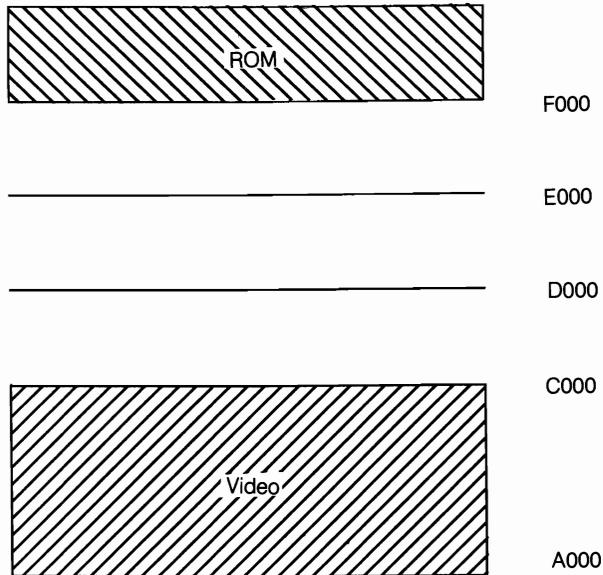
**4-2** The page frame for expanded memory generally is installed at one of three addresses: C000, D000, or E000. However, it need not use these exact base addresses as long as the base address is a multiple of 16K and there is 64K of contiguous memory available beginning at that address.
