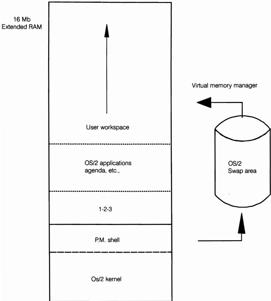
**7-4** A hint of things to come, Lotus 3 also will run under OS/2. In that environment, Lotus 3 uses linear memory as workspace (up to a total of 16K, the limits of an 80286) for even faster operation. Lotus then uses the disk as a virtual memory swap area when RAM is not sufficient for its needs.
