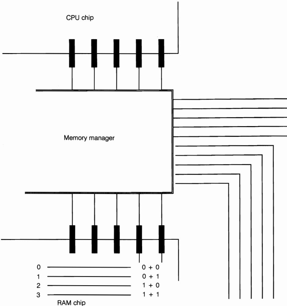
**6-2** This illustration is similar to Fig. 6-1 except that the direct linkage between the CPU and RAM chip address pins has been broken and a memory manager inserted. The memory manager intercepts calls and can reroute them—like call forwarding with your telephone—to different locations. This is the key to accessing 4.0 EMS memory.
