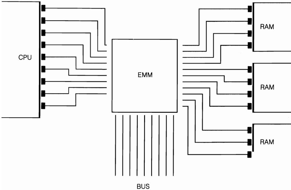
**3-4** In contrast to Fig. 3-3, most well-designed computers today tie only some small part of installed memory (generally no more than 256K) to fixed addresses. The remainder, as shown here, looks to a software memory manager for the allocation that best suits its immediate needs. This allows much more flexibility and more efficient usage.
