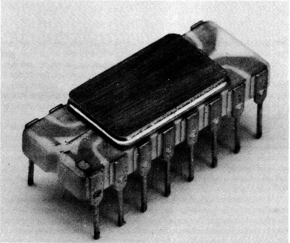
**2-1** Intel's 4004, the world's first microprocessor, is the chip that started it all.
