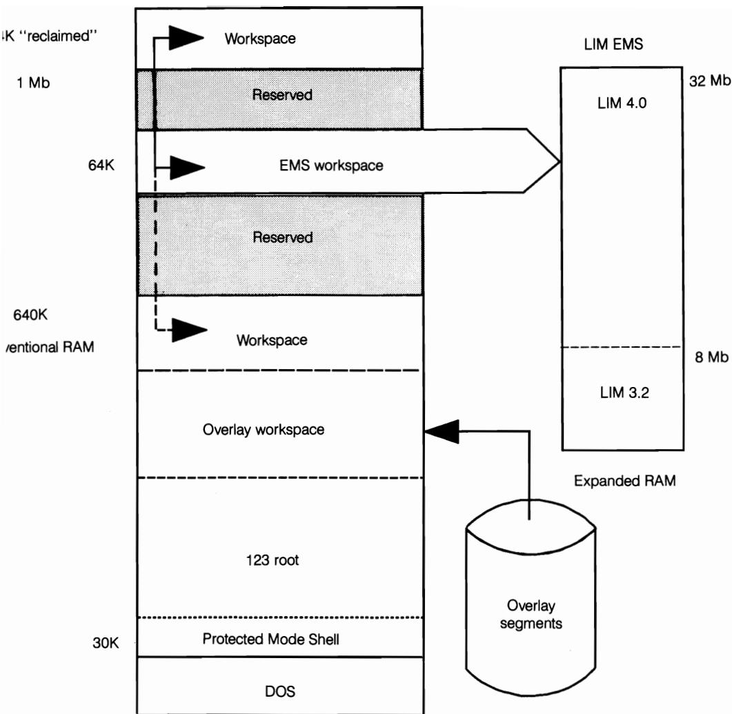
DOS-extended Lotus 3 demonstrates how it can fit on an 80286 (or higher) system with only 1 MB plus expanded memory. However, overlays must be called in from the disk as needed, significantly slowing many operations. Memory shown as "reclaimed" is simply the balance of a full megabyte installed on many computers, 384K of which is above 1024K.
