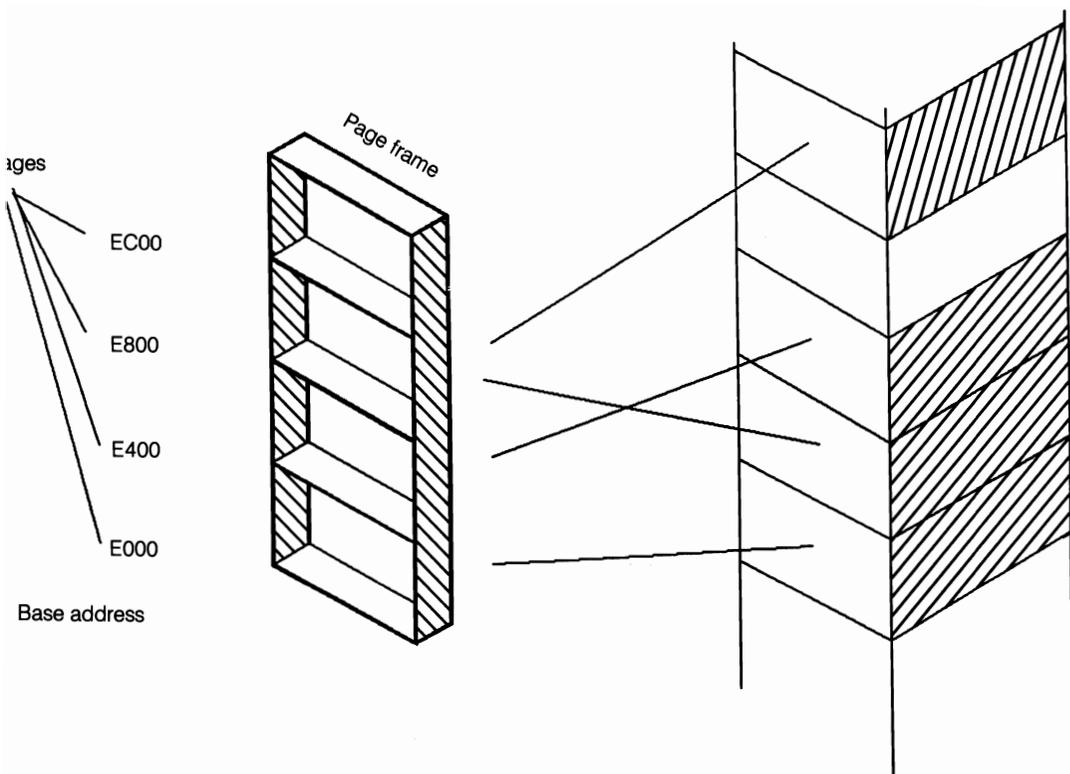
The page frame is divided into four 16K logical pages, as shown here where the base address for the frame is E000.
