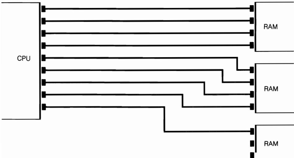
**3-3** In early PCs, specific CPU address pins were hardwired to specific RAM chip address pins or socketing that could support chips answering calls to those specific addresses only. Similar schemes, still found to varying degrees in newer computers, severely limit memory options.
