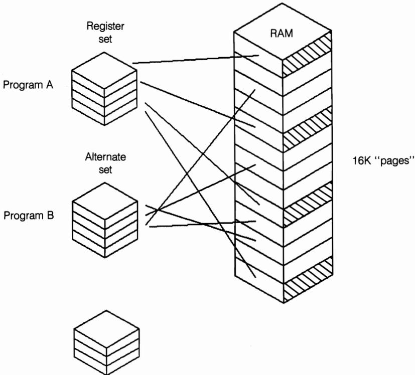
**5-2** The use of alternate register sets is illustrated here. The register set for Program A is pointing to four 16K pages, but an alternate set already is loaded and ready to switch instantly to a different set of pages for Program B, while a third register set is available, if needed. Again for simplicity, sets of only four registers each have been shown here; however, in actual practice, under 4.0 EMS, 64 registers per set are required for full implementation.
