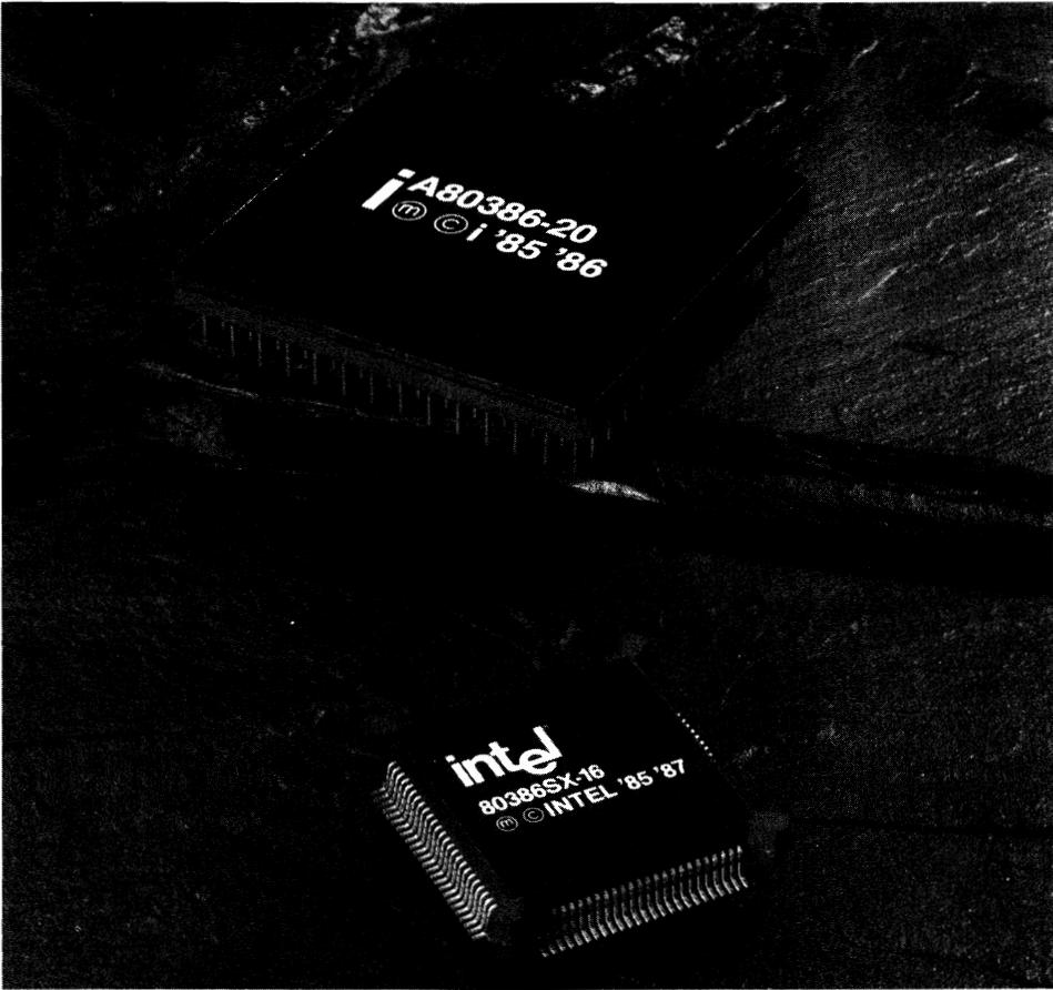
**2-3** Significantly smaller and different in design from the original 80386, the 80386SX offers many of the same benefits, but at a lower cost to systems developers. While only nominally faster than the 80286 and with a smaller address range, it can be used with virtually all 32-bit software written for the 80386.
