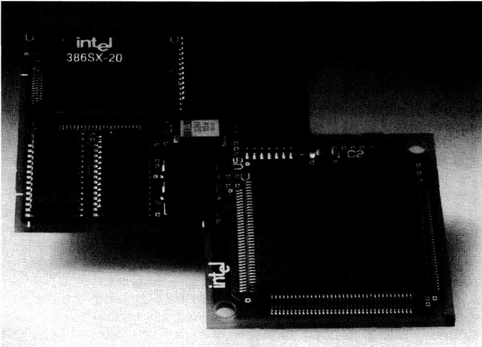
**16-1** Intel's SnapIn 386 module converts 286 PS/2s to genuine 386SXs while maintaining support for 80287 coprocessors. This is only one of several relatively inexpensive plug-compatible upgrade modules that have largely replaced accelerator cards for the 286 market.
