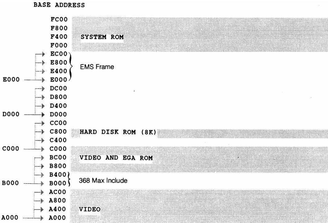
**18-4** This simple form shows addresses above 640K that are known to be in use by various devices. Something like this—either in a hardcopy stored with system documentation or stored for easy access in your computer—can be invaluable in preventing crashes and reducing downtime when you are installing new hardware (or software on 386 systems). Shading can be used effectively to mark out definite off-limits areas, but should be used sparingly to allow for changes.
