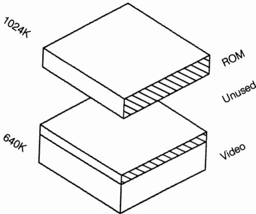
**1-2** Of the original 384K set aside for system use, only the top 64K and the bottom 128K actually were assigned for specific usage (the top for ROM and the bottom for video). Of that latter 128K, many monitors needed no more than the 32K at the top of the block. That left as much as 96K contiguous to the 640K set aside for users completely wasted, along with 192K in the middle. Over the years, system usage of these areas has changed, but there still is much unused space above 640K.
