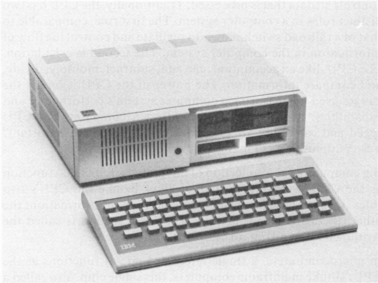
Pictured is the enhanced PCjr System Unit with the internal, half-width minifloppy disk drive and the infrared-linked keyboard. (Photo courtesy of International Business Machines Corporation.)
