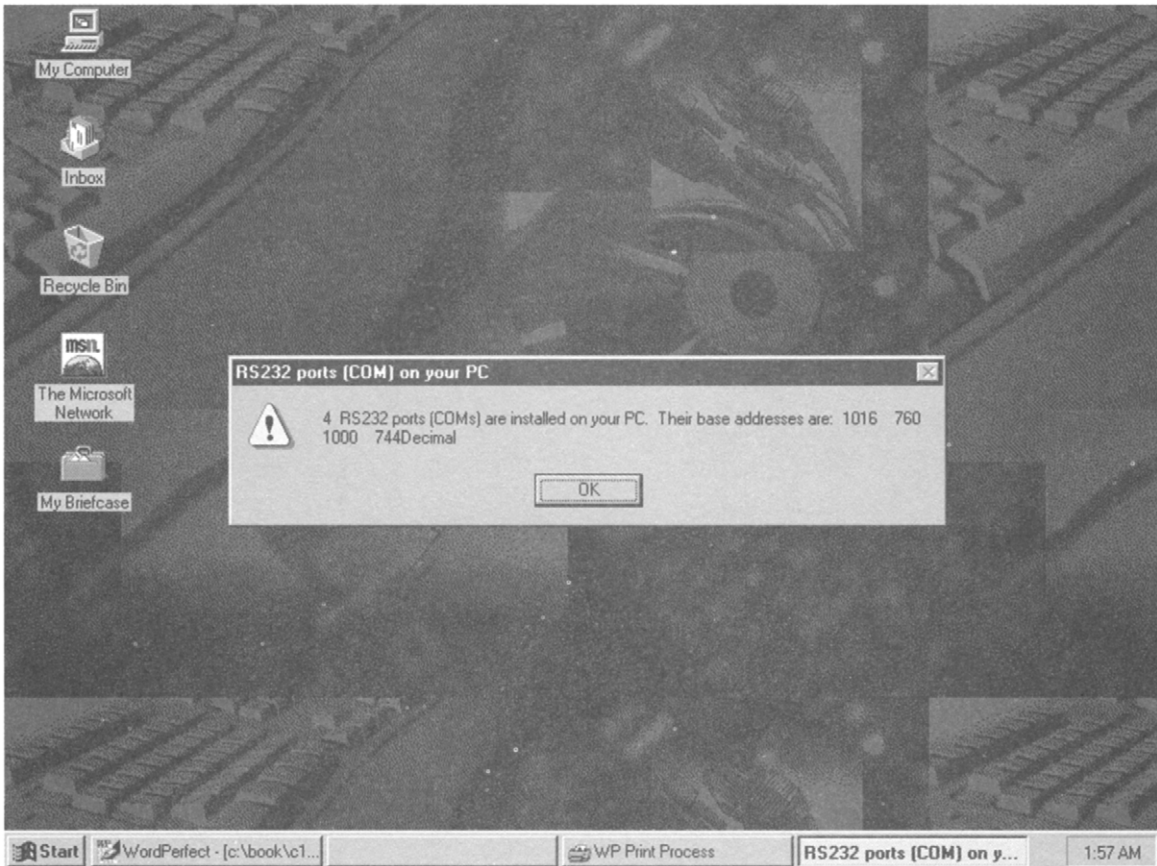
Figure 3.6 Report of the number of RS232 ports installed on a PC by the VB3 driver
