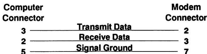
FIGURE 8-5 TXD/RXD Signal Wiring
