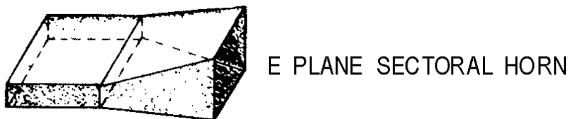
Figure 1-44A.—Waveguide horns. E PLANE SECTORAL HORN.
