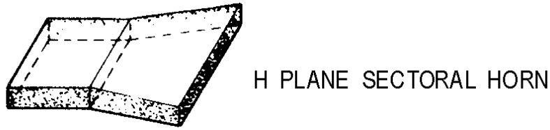
Figure 1-44B.—Waveguide horns. H PLANE SECTORAL HORN.
